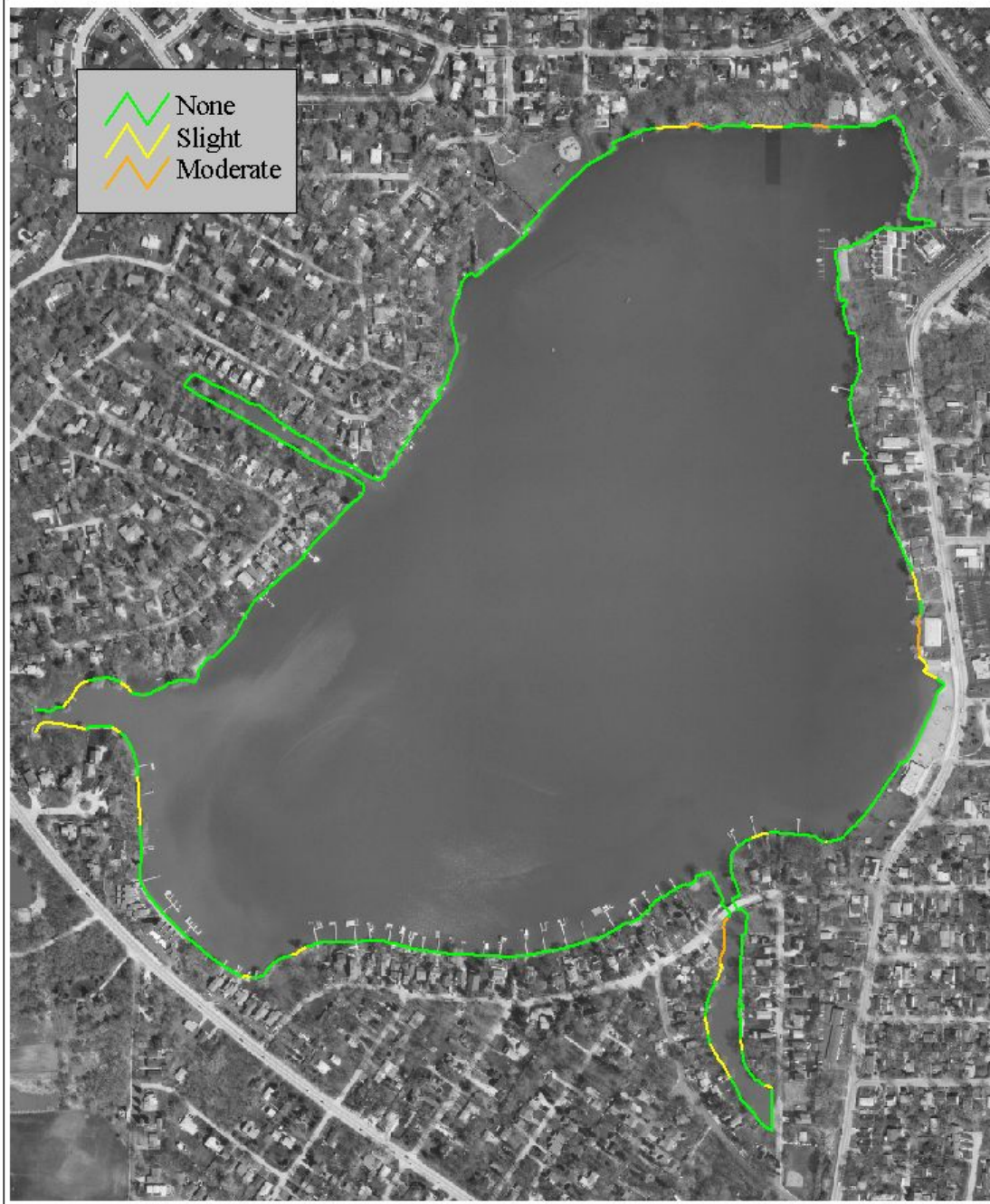
Figure 3. 2002 shoreline erosion on Diamond Lake.
